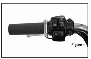
Route the wires from the dual button handlebar control bracket neatly along handlebar into the top fork tree area or inside the handlebar into the top fork tree area. From there run the wire assembly under
